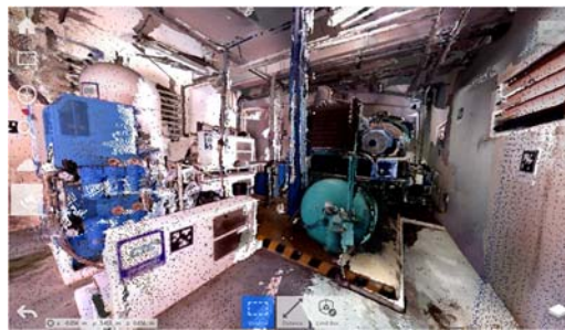
Figure 9 3D point cloud of a crowded mechanical room, created with the handheld scanner
