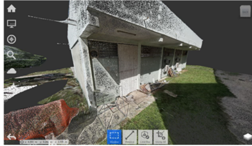
Figure 8 3D point cloud of the exterior of a facility, produced from pictures of a cell phone
