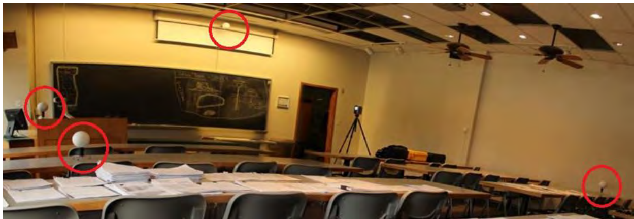
Figure 4. Targets set for laser scanning in the classroom to be retrofitted into a BIM lab.
