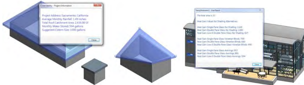
Figure 10: Plug-ins that calculate the size of a rainwater cistern based on location and roof area (Ethan Barley, Andres Lin-Shiu, and Tyler Tucker) (left) and display the heat gain of different types of windows with and without shading (Chris Daubert, Ty Harrison, and Andrew Reego) (right). Spring 2012.
