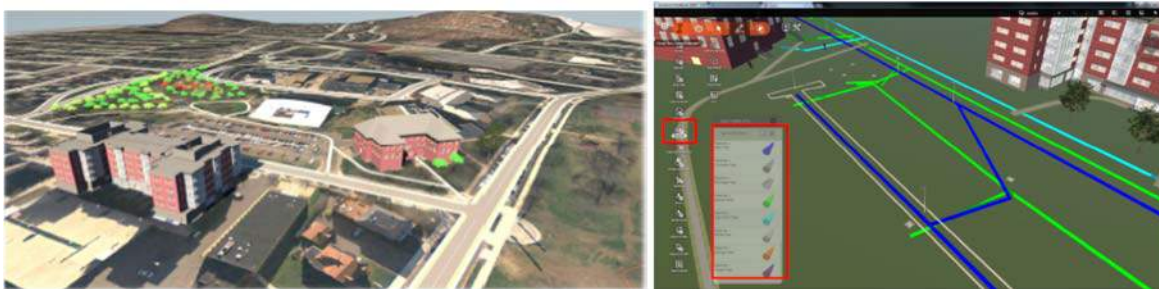
Figure 6 Site-Building Integrated model with underground utilities
