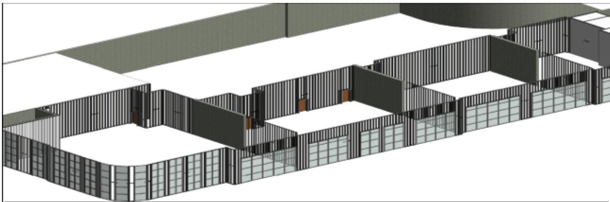
Figure 3: BIM light gauge metal framing 3D view
